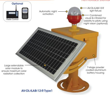
Avlite's low intensity LED obstruction light complete assembly is a self-contained, solar powered obstruction light designed to comply with ICAO LIOL Type B requirements.
