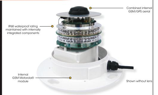
A selection of Avlite lights are available with GSM Cell-Phone Monitoring. This is a cost effective option giving operators remote control over flash code and intensity settings as well as other features for GSM-enabled lights. The system can also be configured to send out warning SMS text messages to designated cell-phone numbers.
